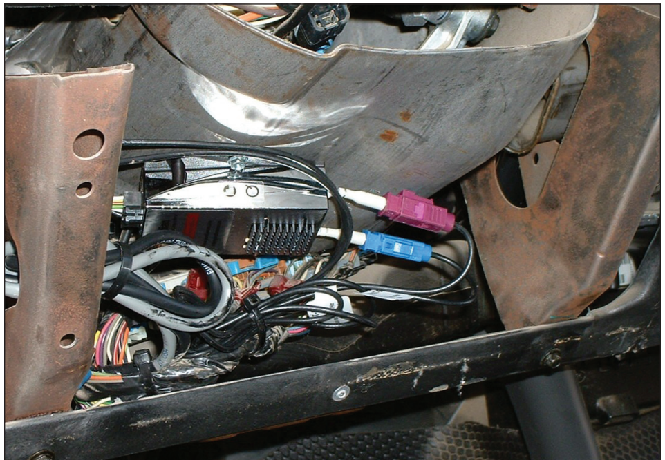
A GPS unit installed under the dashboard of a service truck.
